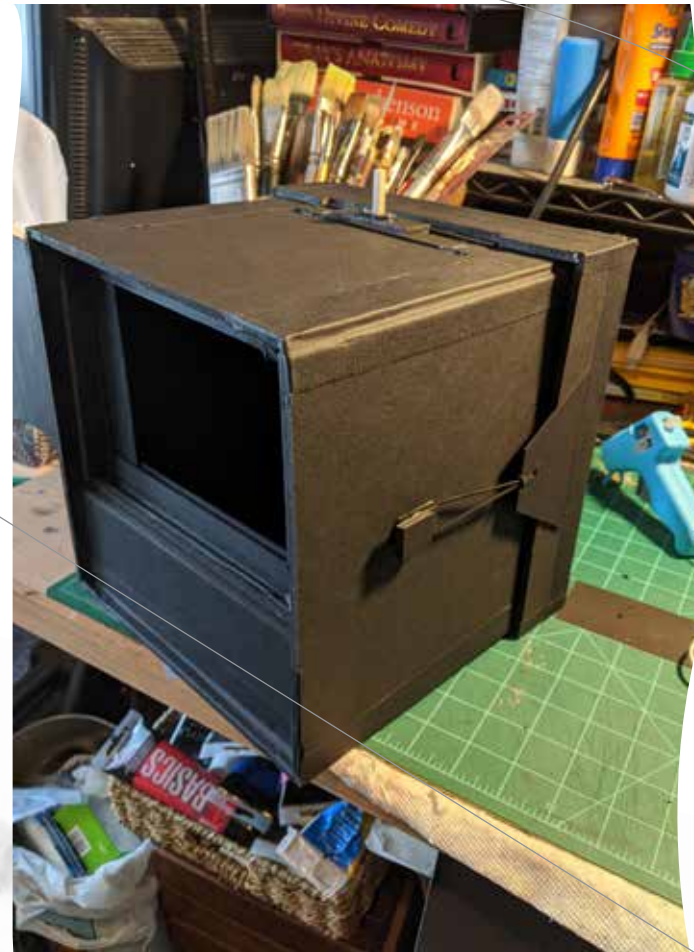
TOP RIGHT: A falling-plate magazine pinhole camera that holds 8 film-holders/plates. I built it out of foamboard.
