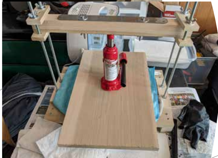
ABOVE: Homemade printing press using a small 2 ton tire jack for small prints, build from hardwoods in my apartment studio.
